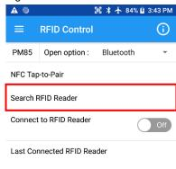
3. When desired RF851 name appears, stop searching by tapping **STOP** and select the name Figure 25 Searching RFID reader
