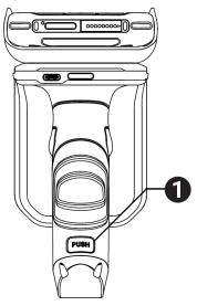
2. Remove the battery and replace it
