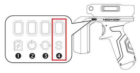
Read RFID tags after pairing the RF851 to your PM85. To read RFID tags, aim the tag and then press the trigger button of RF851 or tap the **Read RFID Tag** button on the screen.
